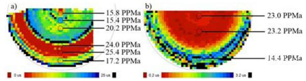
Figure 3: The MCLT images and oxygen content after thermal treatment. The number in the figure refers to the Oi content (PPMa). a) resistivity of 2.2 Ω·cm; b) resistivity of 1.1 Ω·cm.
